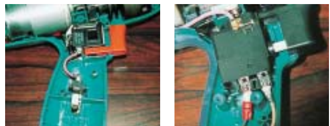
Soldered connections (left) have been replaced with screw-fastened connections (right) that facilitate disconnecting, reconnecting, and environment-friendly disposal processes.
