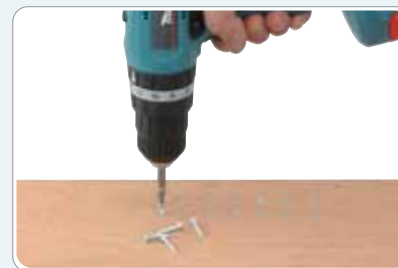
Drove \phi 3.5 \times 22 screws in Lauan.
