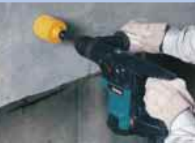
Masonry drilling with core bits
