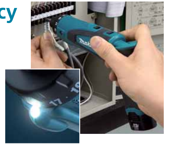
Blinking of LED job light advises the user to recharge the battery.
