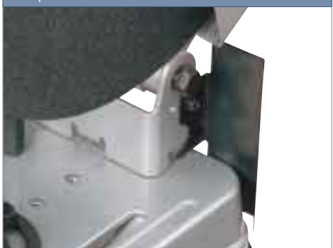
can be adjusted at 3 different positions and at any angle from 90° to 45°
