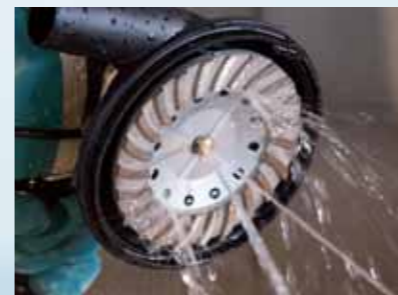
4 Water supply holes
